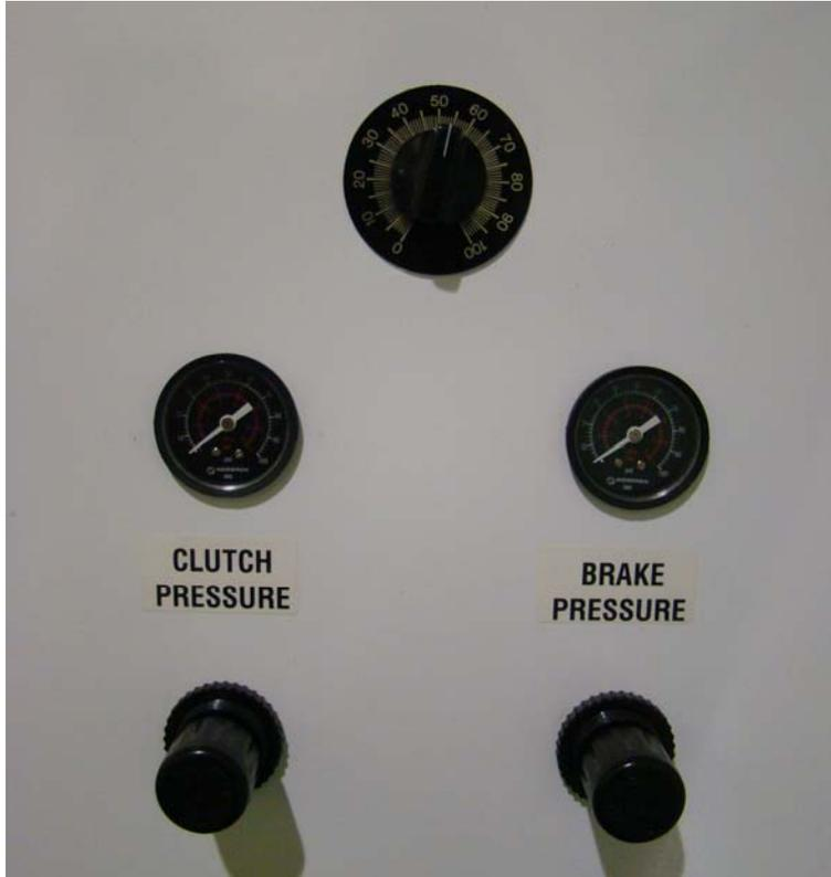
The **dial 0-100** controls the winding rate of the bowls. The faster the wire is fed in the CS327 machine the higher this number needs to be.
