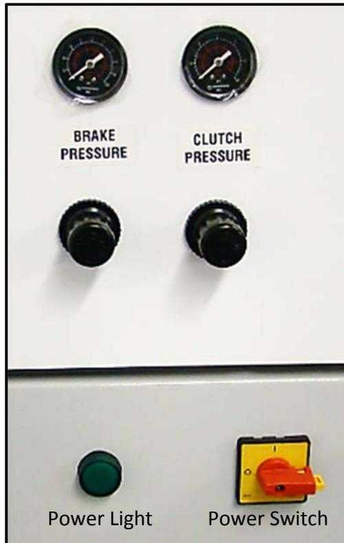
**Break Pressure** – This controls both the brake pressure and the main air on the manifold. You want to set this gauge low enough that the bowl does not slam to a stop causing the wire to spin and tangle up in the bowl.
