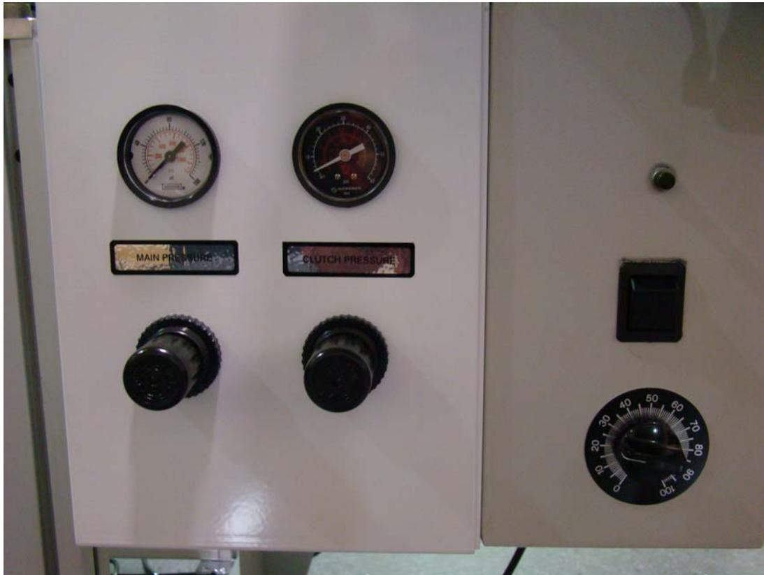
**Main Pressure** – This controls both the brake pressure and the main air on the manifold. You want to set this gauge low enough that the bowl does not slam to a stop causing the wire to spin and tangle up in the bowl. However if you set this gauge too low the shuttle will not be fast enough to switch between the bowls. If it is not fast enough you will get wire jams in the CS326.
