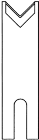
123237 Cut off blade, tangential V. This blade has higher strength than blade 136064, but causes more deformation to large wires due to not having a relief.
