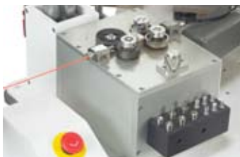
Closed Loop Servo Wire Feed System* ensures length accuracy
