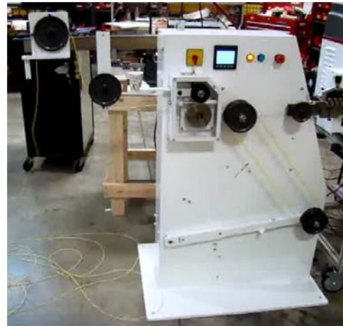
PF-11 Pre-feeder for loose bundle wires.
