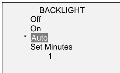
Select **Off** for the backlight to be off upon powering on the tester.
