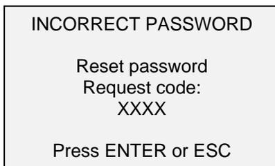
To re-enter the password, press **ESC** to exit to the home screen. Then, access the desired function and enter the password again when prompted.
