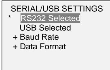
Select either RS-232 or USB input (output is always simultaneous through both the USB and RS-232 ports). Communication settings are permanently set to the following:
