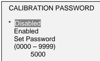
To set the password, select **Enabled**, then **Set Password**. Use the **UP** and **DOWN** keys to increment and decrement the value, from 0 to 9999. When the desired value has been selected, press **ENTER**, then **ESC** to exit the sub-menu.
