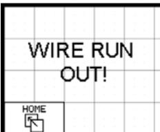
Material has run out. Reload new supply to proceed.
