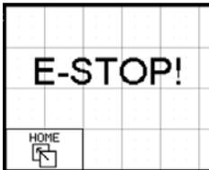
**E-Stop** switch is depressed. Rotate clockwise to proceed
