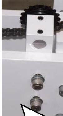
**Adjustment sprocket screws**
