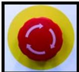
**EMERGENCY STOP:** Depressing this button will deactivate all power from the machine controls. Rotate clockwise to release. **DO NOT PULL.**
