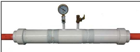
The Blue Diamond Barbed Coupler is a compression fitting and must be installed using a Hydraulic or Mechanical coupling press. The coupling press ensures the HDPE conduit ends butt up against each other to enhance cable blowing. It also compresses the coupling forcing the barbs into the duct, ensuring great pull out strength and sealing capacity. Long haul telecom contractors prefer barbed compression couplings because of their reliability and ease of
